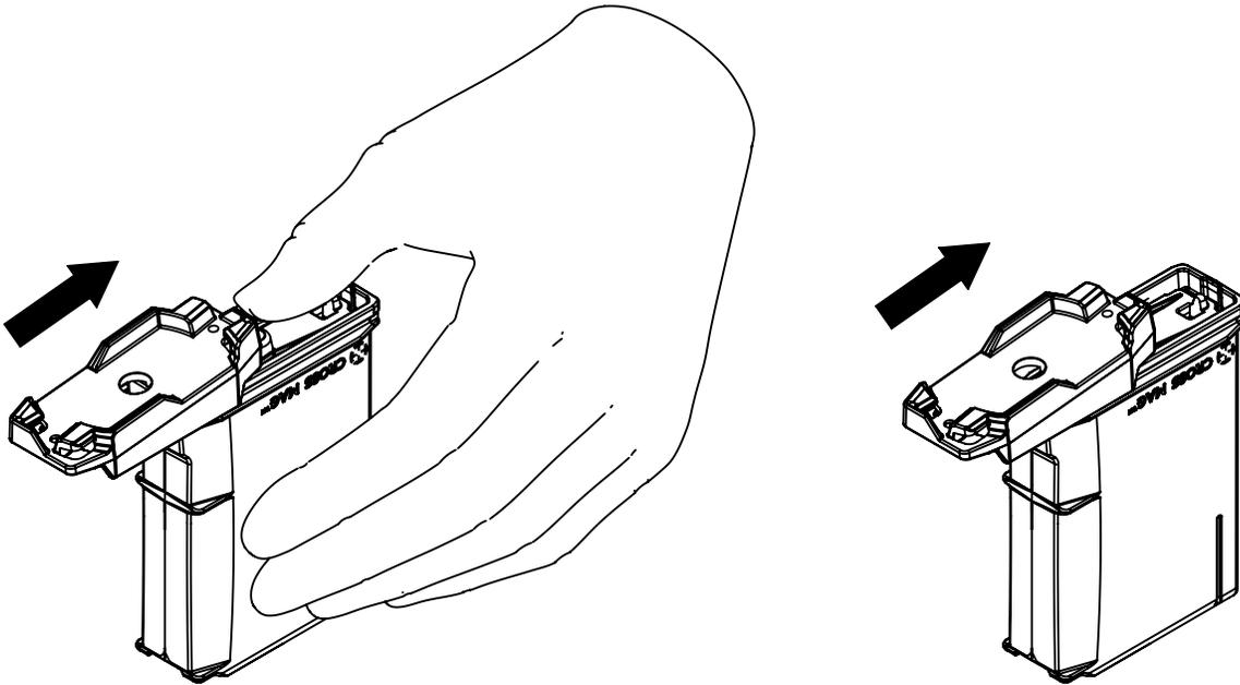
**STEP 2:** Fully slide the floor plate on to the mag until the spring plate and floor plate engage.
