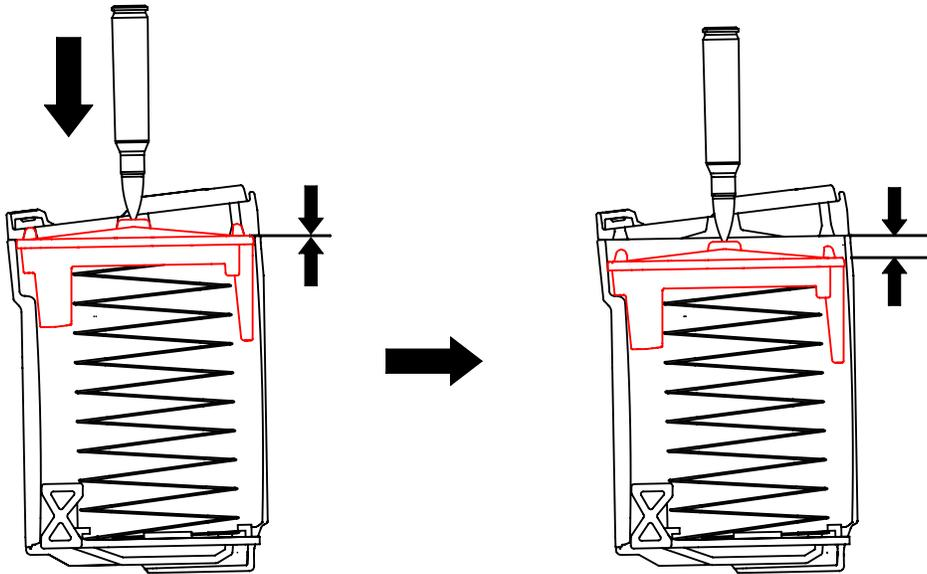
**STEP 2:** Slide the floor plate off the mag, ensuring the spring plate does not eject by pressing a thumb down during the removal of the floor plate.
